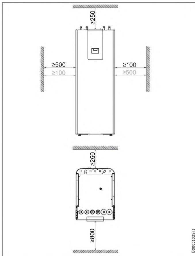
The minimum side clearances can be swapped between left and right.
