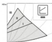
The pump reduces the delivery head by half when the flow rate in the pipework decreases.
