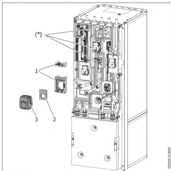
(\*) Pipe assembly inserted
