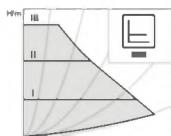
The control system keeps the set delivery head constant, irrespective of delivered flow rate.
