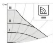
The pump runs at three preset fixed speed levels (I, II, III).
